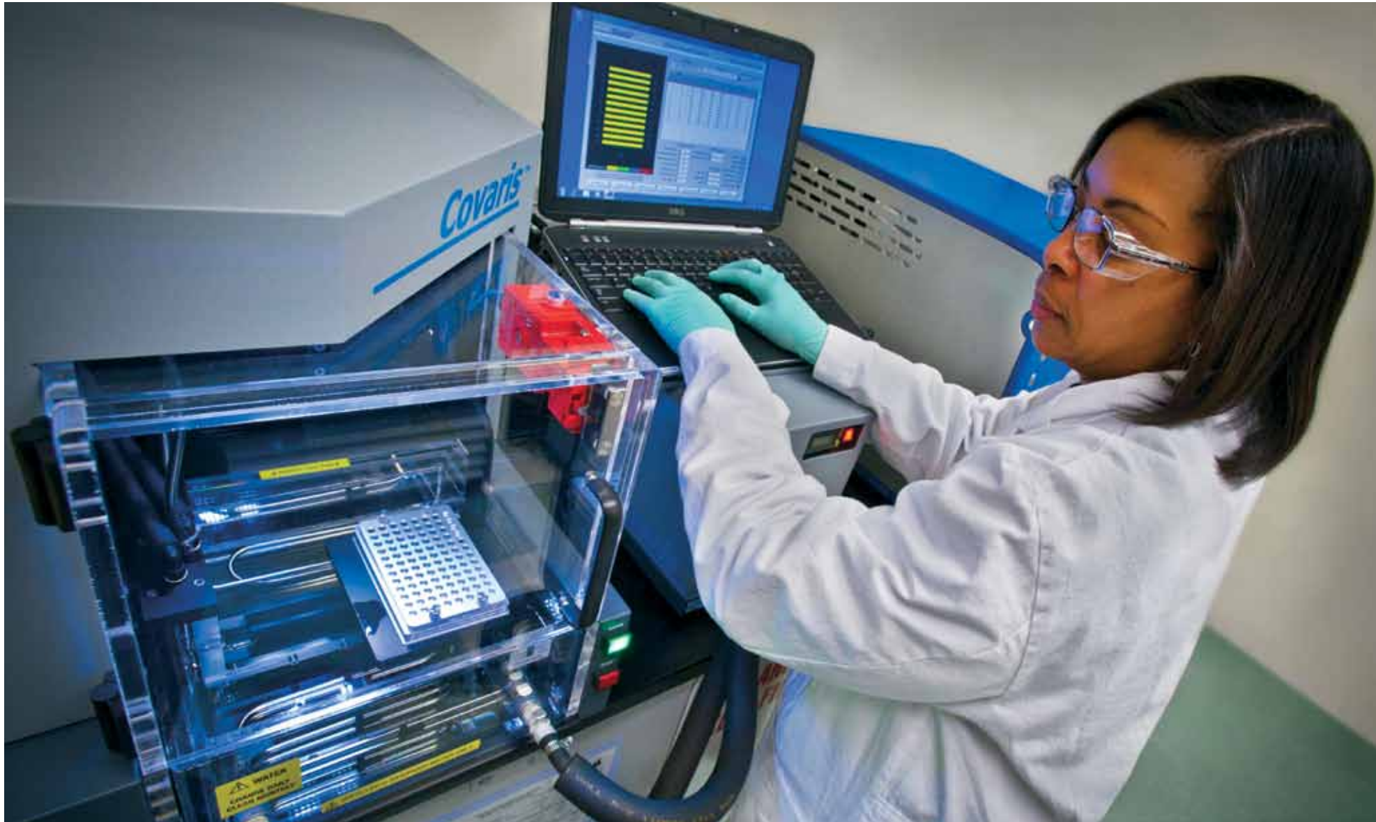
The sonicator shears DNA fragments for library creation.
