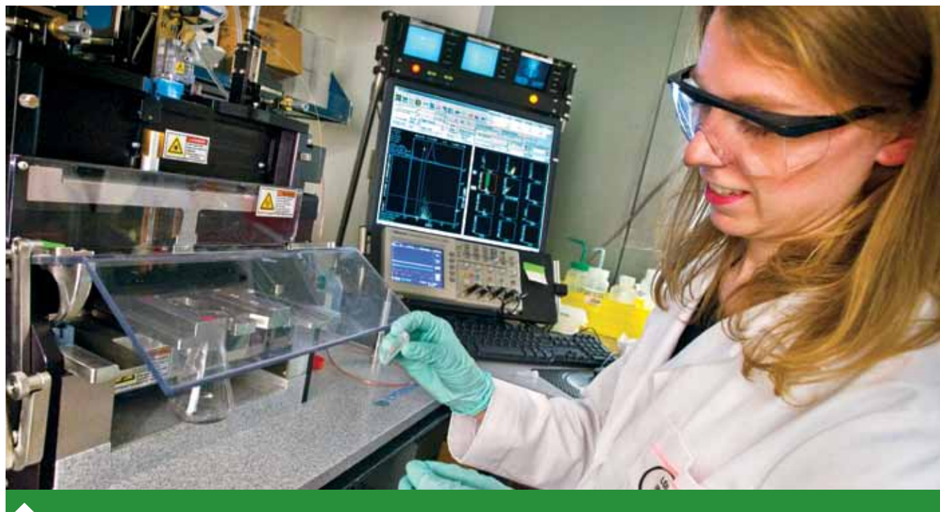
The cell sorter separates single cells in suspension based on their expression of fluorescent reporter genes.
